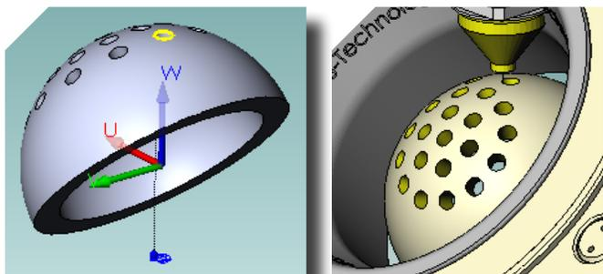
Specialized multi-axis Ruled features are used for operations that require continuous rotation. The match lines contained in the feature automatically control the synchronization of the wire throughout the cut.
